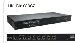
HDMI Splitter 1x8 over HDBase-T/70m
