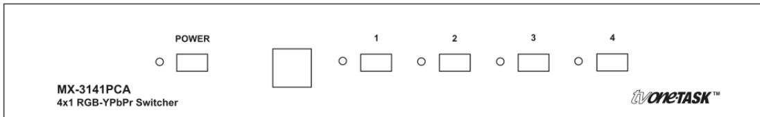
The front panel contains the power switch and LED Power Indicator, the Infrared Sensor window and the four input selectors plus LED indicators that show which input has been selected.
