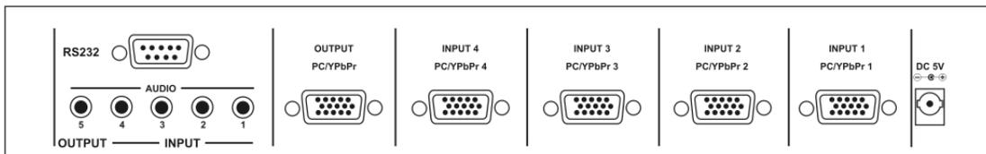
From left to right, the rear panel features the RS-232 connector and five 3.5mm type connectors for the Left and Right analog audio channel I/O.
