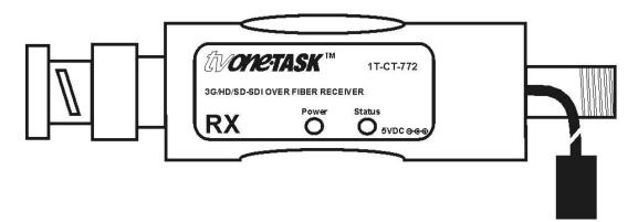
At the remote location, connect the Fiber Optic cable to the Fiber input of the Receiver.
