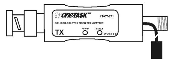
Connect the SDI source device's output directly to the 1T-CT-771 Transmitter via the BNC connector. (Use of an intermediate cable is permitted after you have verified operation of the entire path without an intermediate cable. This ensures that the system is working properly and removes the variable of an intermediate cable that is too long or of poor quality. Once the system's functionality is verified, you can attempt to use an intermediate cable.)
