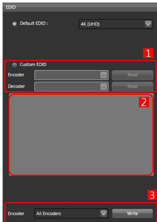
Figure. 31-7 Encoder Device Setup – EDID Setup
