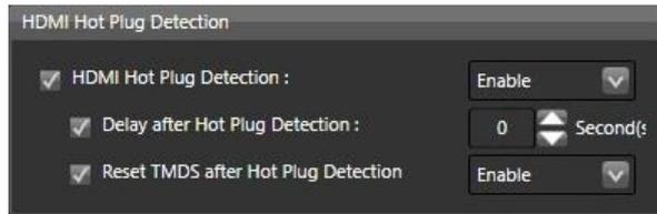
Figure. 31-4 Encoder Device Setup – HDMI Hot Plug Detection
