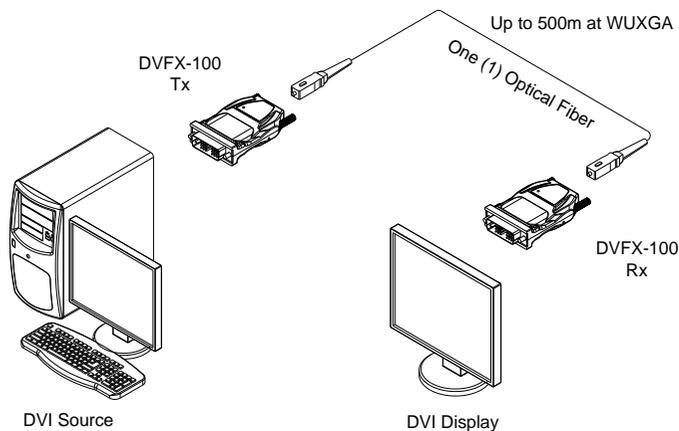
Figure 1 – Connection Diagram of Optical DVI Extension Module
