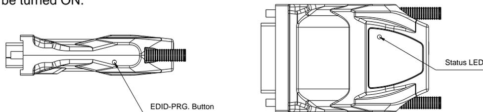
Figure 5 – Position of EDID-PRGM. button and Status LED
