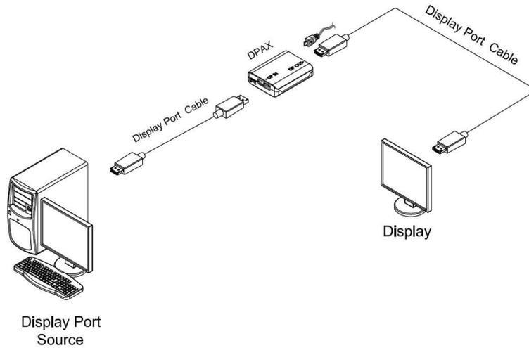
Figure 2 – Connection of DPAX with Copper cable
