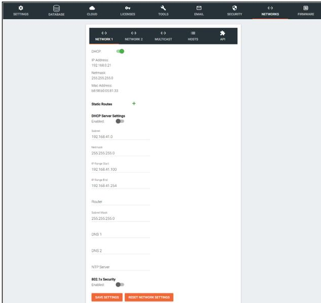
Network 1 corresponds with Ethernet Port 1 of the AT-VGW and can be set between static IP, DHCP, and DHCP server. If set as a DHCP server, a range of IP addresses must be set so it can assign IP addresses for anything else connected to the network.
