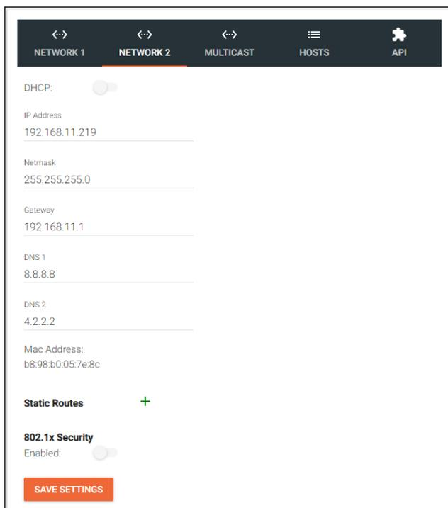
Network 2 corresponds with Ethernet Port 2 of the AT-VGW and can be set between static IP and DHCP.
