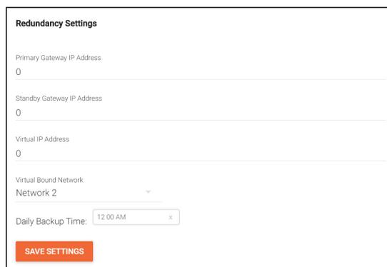
**NOTE:** Both gateways must be connected to the network using the same Ethernet port on the units. If the primary gateway is connected to Ethernet port 1 then the backup gateway must also be connected to the network using Ethernet port 1.
