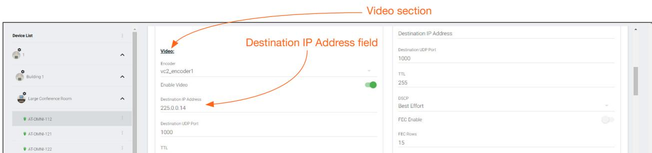
11. Locate the **Destination IP Address** field and delete the value in this field.
