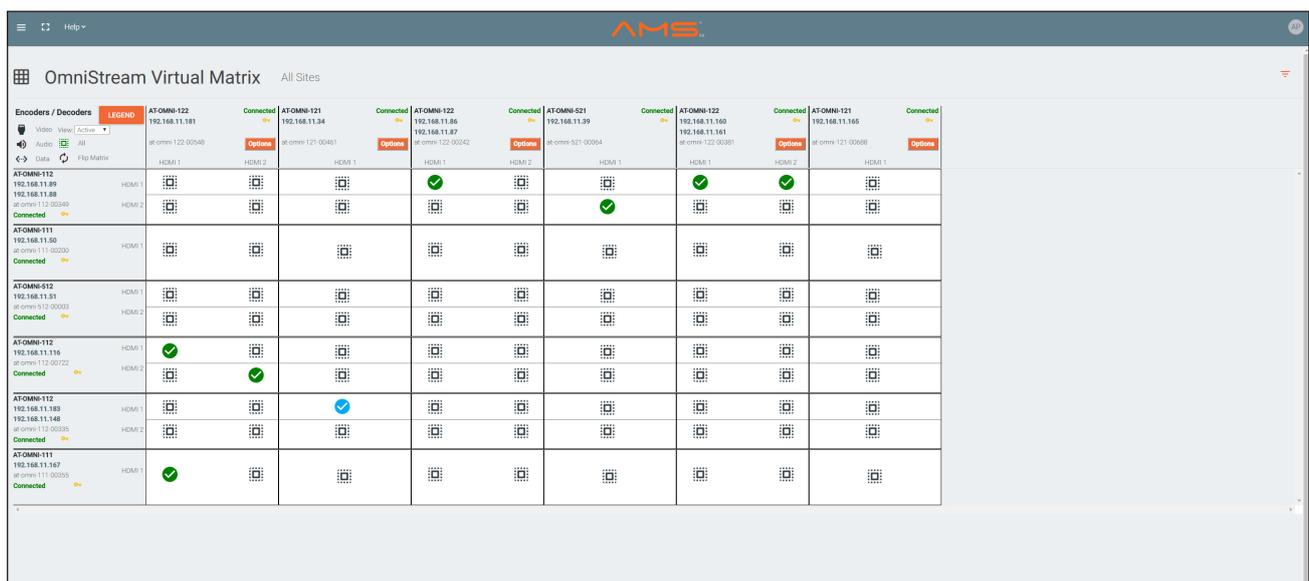
The screenshot displays the 'OmniStream Virtual Matrix' page. It features a table with columns for encoder models and their IP addresses, and rows for different HEM (Host Encoder Module) units. The table shows connection status for various AT-OMNI-111 and AT-OMNI-112 encoders across multiple HEMs.
