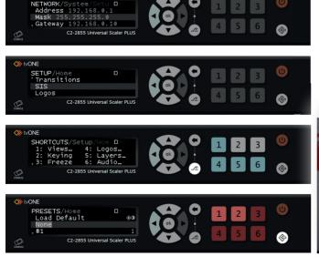
Using the 2 step preset setup configurations can be stored to enable quick screen changes at the touch of a button.
