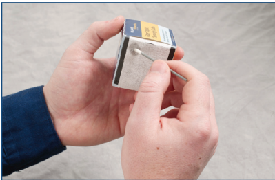
Touch the swab to the wet spot on the wipe for 3 seconds to absorb a minimal amount of solvent. A damp swab works better than a wet one. Applying solvent from the pen directly to the swab will likely result in excessive solvent.
