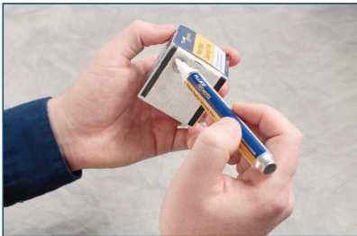
After pulling a clean wipe from the cube, apply a small spot of solvent to the starting edge of the wipe.
