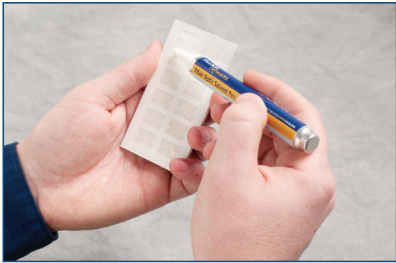
After removing one plastic cover, apply a small spot of solvent to the starting corner of the cleaning zone.
