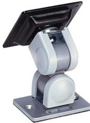
The FPMA-DTBW200 is the connection between toolbar and screen. This mount fits all screens up to 24" and a maximum weight of 10 kg. The mount has the VESA hole pattern 75x75mm. If VESA100 is needed, adapter item FPMA-VESA100 needs to be purchased additionally. If your screen has different VESA hole patterns, please contact us.
