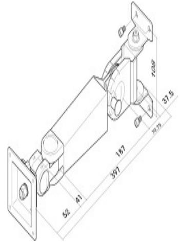
The NewStar LCD/TFT wall mount, model FPMA-W400, allows you to mount a flatscreen to the wall.
