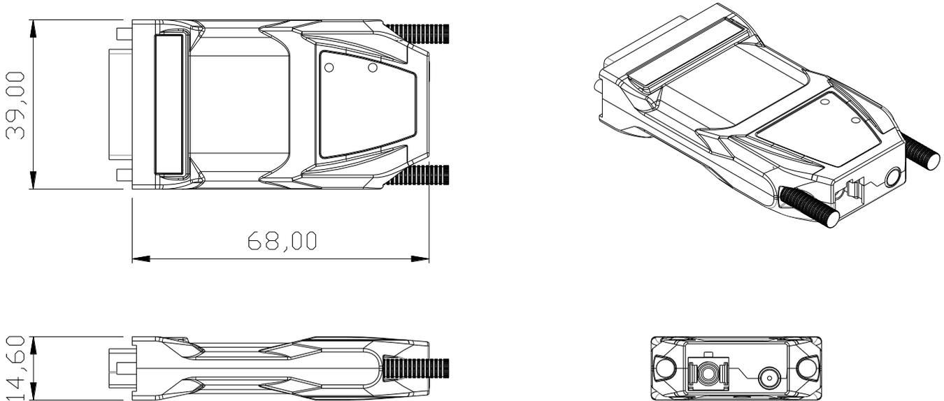
Note: The transmitter, DVFX-110-T and the receiver, DVFX-110-R have the same mechanical dimensions.
