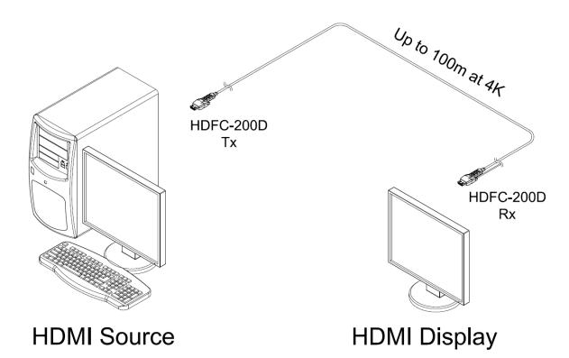
Example: PC to HDMI Monitor Set-up Source: DVD, PC, Set-top box, Console Display: UHD TV, Projector, 4K monitor
