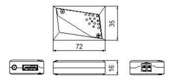
Note: The transmitter, HDFX-250-T and the receiver, HDFX-250-R have the same mechanical dimensions
