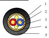
1. Conductor 32 x 0.10 mm Bare Oxygen-free Cu
