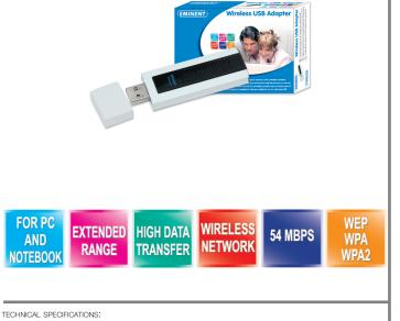
TECHNICAL SPECIFICATIONS: Interface: USB 2.0 Antenna: Internal Intellective Antenna Wireless standards: IEEE 802.11b/IEEE 802.11g Frequency: 2.4 ~ 2.4835GHz Media Access Protocol: CSMA/CA with ACK Transmit power: 17dBm Security : WPA/WPA2, 64/128/152 BIT WEP, TKIP/AES Dimensions: 80 x 27 x 10 mm
