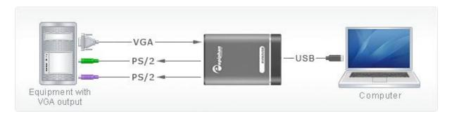
The product provides a simple, portable, lightweight and rapid means of conveying VGA images from host machines to a laptop and simulating the laptop's keyboard and mouse outputs. This allows administrators and technicians to quickly and easily connect to—and administer— headless machines without hassles, without having to use a network.
