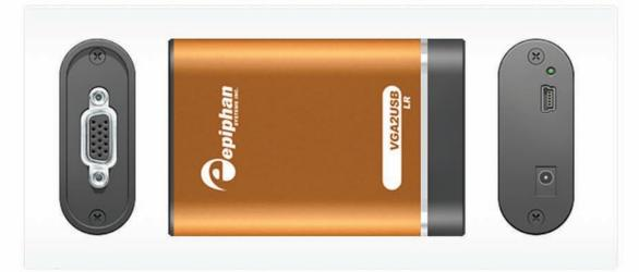
VGA2USB LR is a frame grabber designed with price and versatility in mind. It's priced significantly lower than topend devices such as the VGA2USB HR or Pro, yet shares many features with them. This includes Epiphan Systems' lossless compression technology and on board RAM. The VGA2USB LR is able to capture lossless images with resolutions of up to 1280x1024 at frame rates of at least 30fps.
