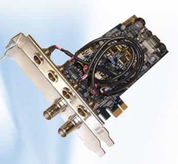
The Osprey 710e HD features a high-definition SDI video input, with an additional SDI/BNC monitor out to facilitate workflow. In addition to 8 channels of embedded SDI audio (4 stereo pairs), the Osprey 710e HD includes 4 stereo pairs of AES/EBU digital audio inputs implemented across mini XLR connectors, providing maximum audio flexibility.
