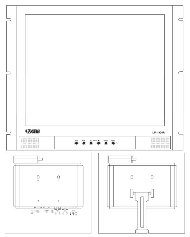
An AC Adapter is included with each unit. Insert it into the holder located at the top, rear of the unit. Connect its DC cable to the connector labeled **DC +12** and then connect the included AC cable to the AC Adapter. Connect all input cables to the unit and lastly connect the other end of the AC cable to the AC power source.
