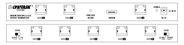
Connect the HDMI source device's output to the HDMI IN connector of the 1T-CT-637 Transmitter, using an appropriate HDMI cable of no more than 10 meters (33') in length.
