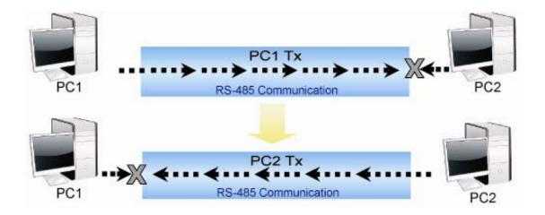
Auto Carrier Sense (ACS<sup>TM</sup>) technology will check the status of RS-485 communication bus. If the bus is idle, it starts transmission. If the bus is not idle (some data flows in the bus), then it will postpone the transmission of UART until the bus is idle. Due to the reduction of TX/RX packet conflicting on RS-485 one-way traffic bus, it will enhance better system performance and RS-485 communication ability.
