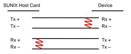
2-Wire RS-485 working model with termination resistor:
