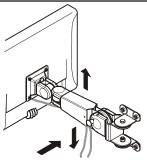
d. Move arm upwards & downwards and make sure knob have wedged into slot. Release support on LCD monitor.
