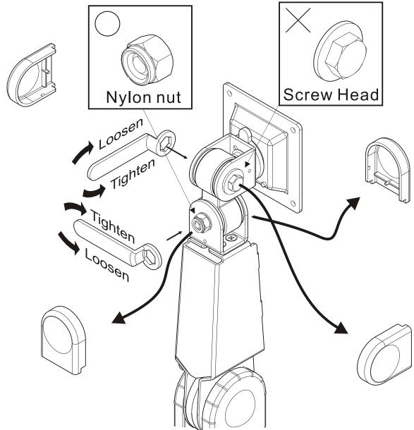
When assembling the arm with monitors of differing weights, you may find that the tension of the universal joint needs to be adjusted to ease movement or to maintain the desired monitor position. If so, adjust as follows:
