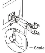
c. Pivot arm to view angle needed (aim at triangle mark) then let go of knob.
