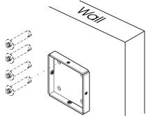
Secure bottom plate firmly to the wall with four expansion screws (not supplied).
