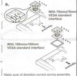
Make sure of direction correct during assembly. (as illustrated)
