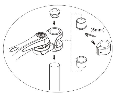
Put axle sheaths into upper and beneath holes of the connection block. Then put the stopper in together with pillar. Adjust the level of high to the most comfortable view. Secure it with screw and then put in the plug.
