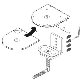
Use 6mm Allen key to secure the cranking unit to the bracket with at least two bolts.(For desk 15~100mm thick, over 30mm is suggested.)Use 4mm Allen key to secure the pillar & clamp with 4 screws.
