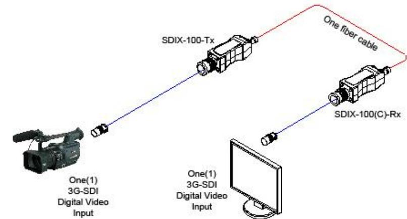
Figure 1 – Fiber-Optic 3G-SDI Extension module, SDIX-100
