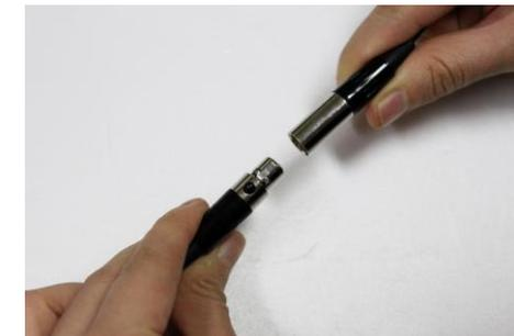
Figure 3 –SDIX-100 with power adapter
