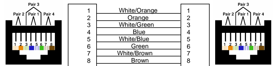
Figure 7 – Wiring Diagram of CAT5 Cable (Direct Type)
