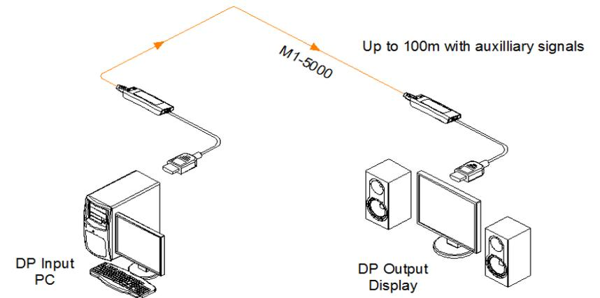
Figure 1 – Optical DP extension Cable, M1-5000
