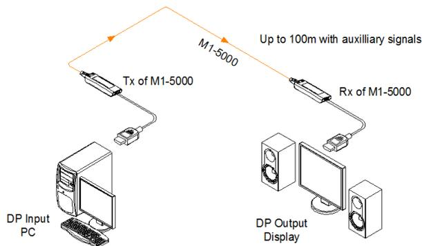
Figure 5 – Whole Connection of M1-5000 Cable
