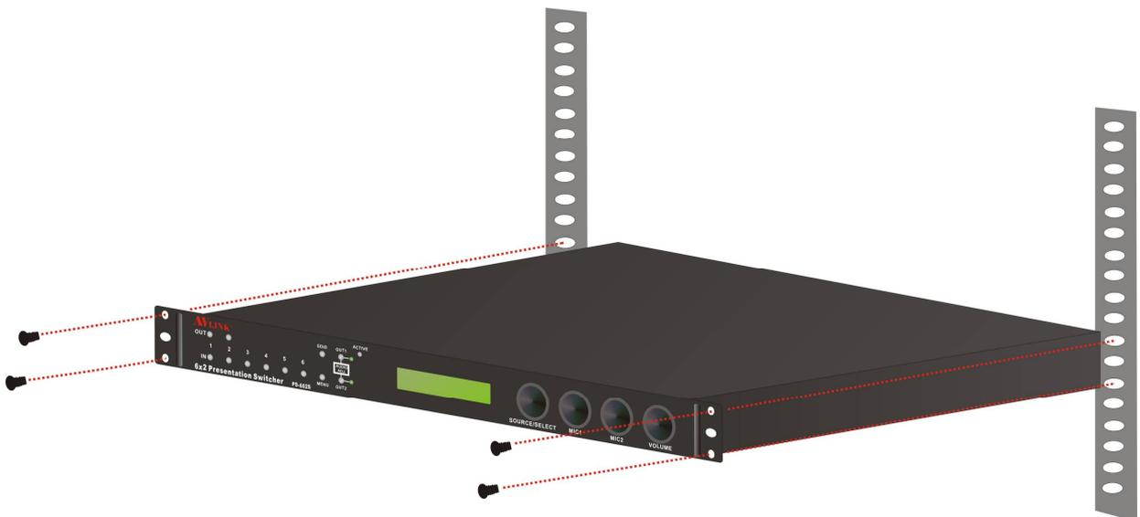
**Figure 4-2 Mount the Switcher in the rack**
