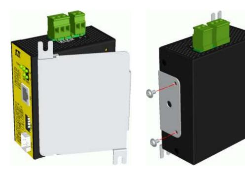
3. Screw the device on a panel and the locations for screws are shown below:
