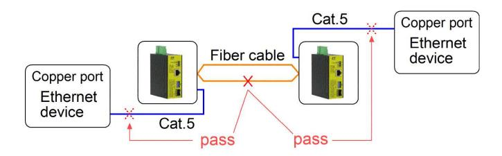
Both Ethernet devices will also detect a link fault on each Cat.5 connection, although the real fault occurs on the fiber connection exactly.
