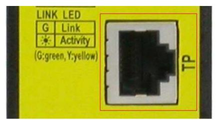
The 10/100/1000 RJ-45 TP port supports the following connection types and distances:
