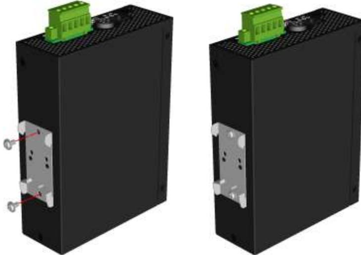
2. Attach bracket to the lower edge of the DIN rail and push the unit upward a little bit until the bracket can clamp on the upper edge of the DIN rail.
