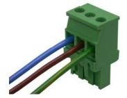
Install the wired plug onto the AC socket properly. For safety purpose, use the provided yellow cap to cover the unused IEC320 receptacle.
