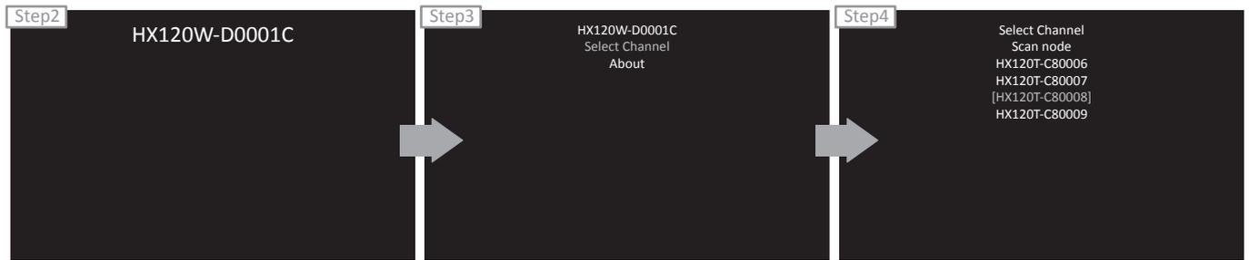
2. The device ID will appear on the screen. To specify the desired device, press **Left** or **Right** button. Once the device has been confirmed, press **OK** to bring up more options.
