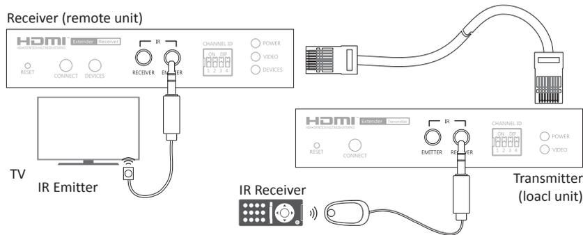
**Caution:** Plug the IR Receiver and IR Emitter into the respective jacks, otherwise the IR sensor on the IR Receiver and IR Emitter will be invalid.
