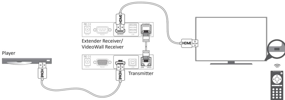
1. Make sure the connected AV equipments and TV/monitors are compatible with HDMI CEC.
