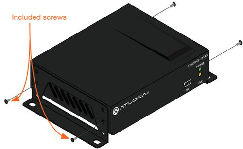
4. Mount the unit using the oval-shaped holes, on each mounting bracket. If using a drywall surface, a #6 drywall screw is recommended.
