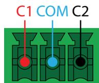
There are 3 connections for the relay: C1, COM, and C2 (Circuit 1, Common, and Circuit 2.)
