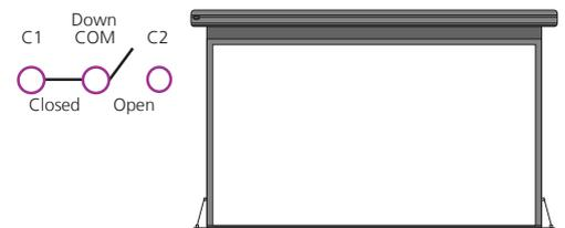
The relay will default to follow the display. When the unit turns on the relay will close C1 and open C2. When the display is turned off and signal is no longer being received C1 will open and C2 will close.
