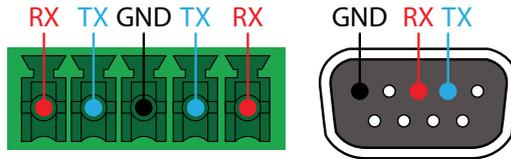
Pin out will be determined by the RS-232 cable and connect as RX (receive), TX (transmit) and  $\perp$  (Ground). Ground will be shared between port 1 and port 2.
