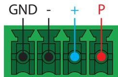
There are 4 connections for the trigger: GND, -, +, and P (Ground, Negative, Positive, and Power).
