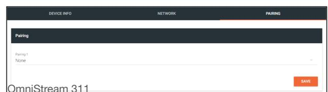
6. Select the unit to pair to from the drop down menu. The OmniStream 311 can pair with up to 7 devices, the OmniStream 324 can pair with only 1. It does not matter which drop down is used on the AT-OMNI-311 as it will assign it to any port.
