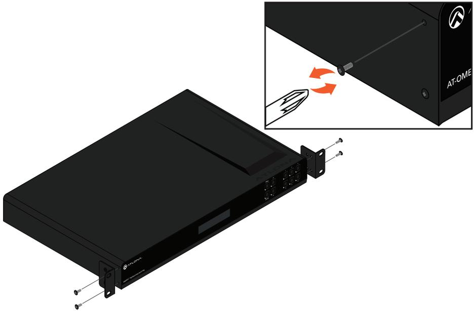
3. Install the OME-PS62 into a rack, using four rack screws.
