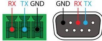
Pin out will be determined by the RS-232 cable and connect as RX (receive), TX (transmit) and  $\perp$  (Ground). Ground will be shared between port 1 and port 2.
