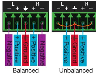
Use a jumper between the negative and ground pins when using an unbalanced connection.
