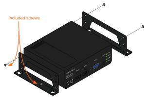
4. Mount the unit using the oval-shaped holes, on each mounting bracket. If using a drywall surface, a #6 drywall screw is recommended.
