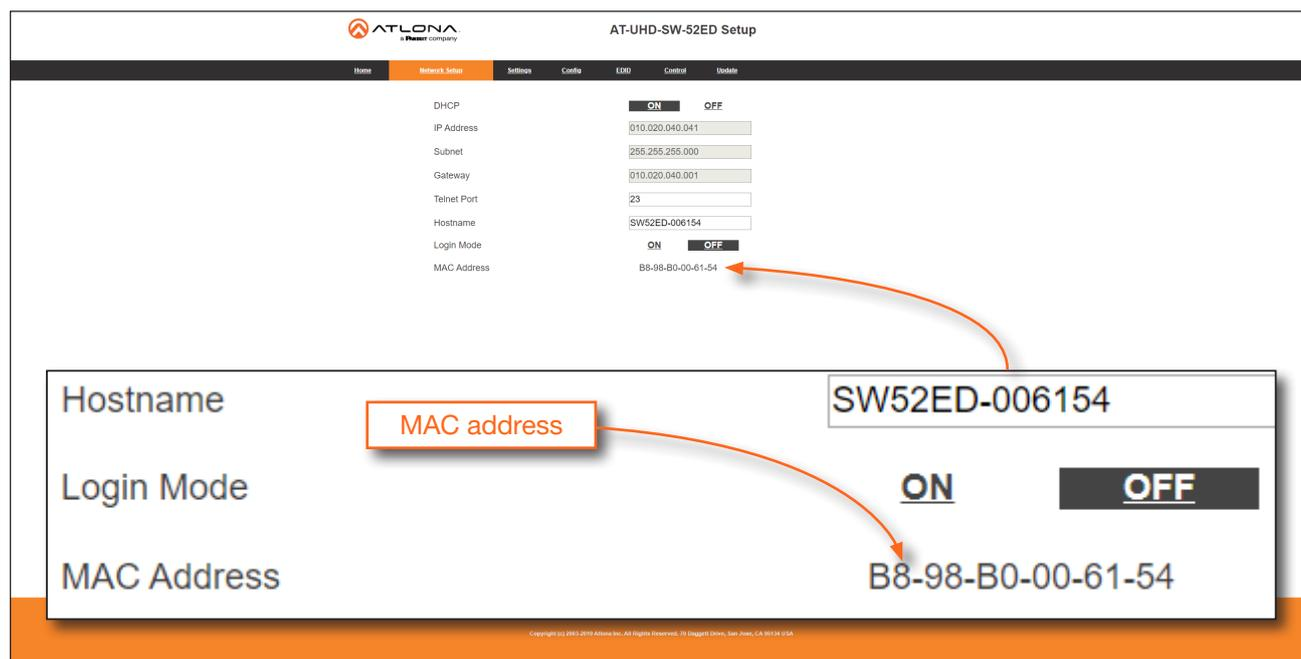
The screenshot shows the 'AT-UHD-SW-52ED Setup' web interface. The 'Network Setup' tab is selected. The settings are as follows:
