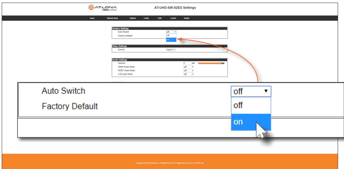
The screenshot shows the AT-UHD-SW-52ED Settings page. The 'System Settings' section has 'Auto Switch' set to 'off'. A dropdown menu is open for 'Auto Switch', showing 'off' and 'on' options. A mouse cursor is pointing at the 'on' option. The 'Factory Default' is also shown as 'off'. The 'Video Settings' section shows 'Source' set to 'Input 1'. The 'Audio Settings' section shows 'Volume' at 0 dB, 'HDMI Audio Mute' set to 'off', 'HDBT Audio Mute' set to 'off', and 'L/R Audio Mute' set to 'off'.
