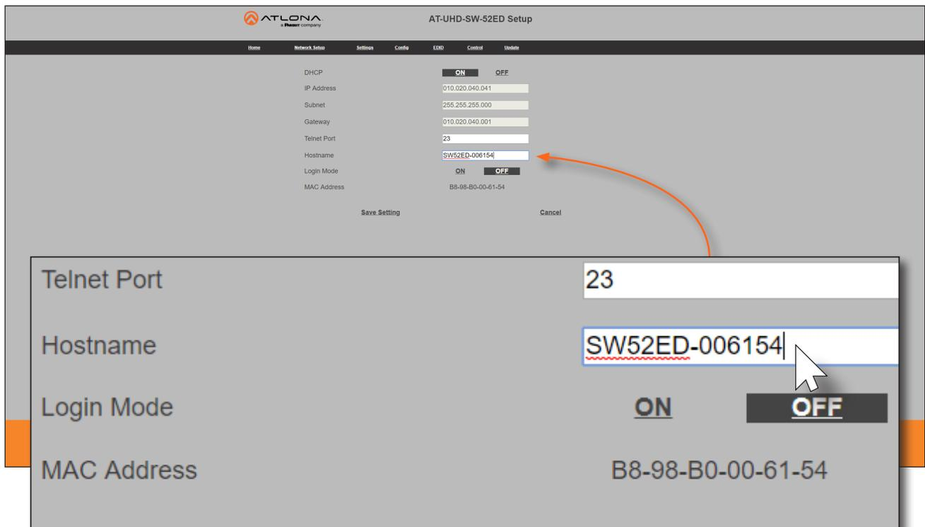
The screenshot shows the AT-UHD-SW-52ED Setup web interface. The main settings area includes fields for DHCP (ON/OFF), IP Address (010.020.040.041), Subnet (255.255.255.000), Gateway (010.020.040.001), Telnet Port (23), Hostname (SW52ED-006154), Login Mode (ON/OFF), and MAC Address (B8-98-B0-00-61-54). A red box highlights the Hostname field, and a mouse cursor is positioned over it. An orange arrow points from the Hostname field in the main settings area to the expanded view below.
