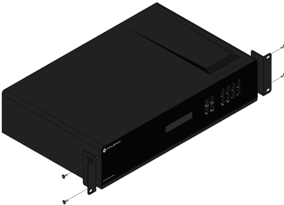
3. Install the matrix into a rack, as shown using the included rack screws.
