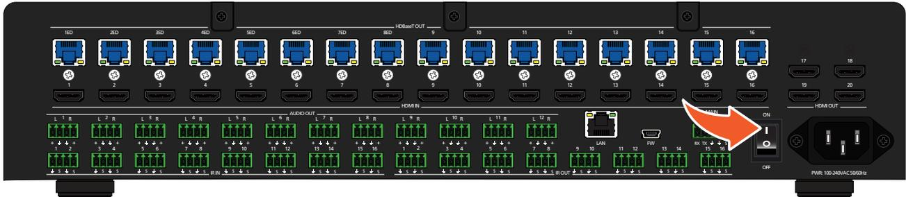
**NOTE:** If the matrix does not power, check to make sure that the power cable, on the rear of the unit, is connected to an active AC wall outlet. Also verify that the **ON/OFF** switch is in the **ON** position.
