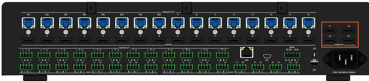
These four HDMI ports are used to mirror (copy) an HDBaseT output signal and duplicate it on any or all of these ports. By default, mirroring is enabled on these ports. However, mirroring can be disabled. When mirroring is disabled, any of the 16 HDMI inputs can be routed to these HDMI outputs, transforming this product into an 16 x 20 matrix switcher. The default mirror settings are listed below
