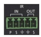
The included IR emitter has two wires: signal and ground. Signal will have a solid line and ground will be blank. The IR emitter will plug into the IR OUT ports.
