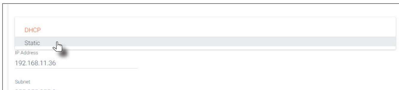
9. Enter the required network information for the decoder in the **IP Address**, **Subnet**, and **Gateway** fields.
