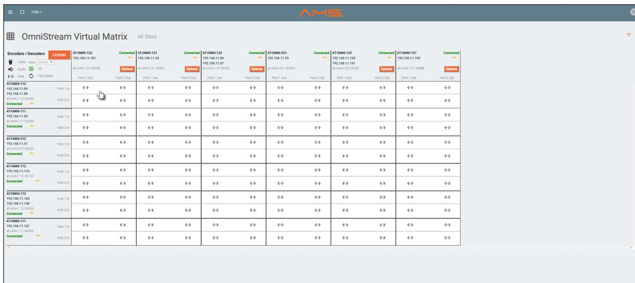
2. Locate the desired encoder and decoder where the cross-connection will be created. In the following example, **Port 1 In** and **Port 1 Out** on the AT-OMNI-112 and AT-OMNI-122 (in the upper left corner of the Virtual Matrix), will be selected.
