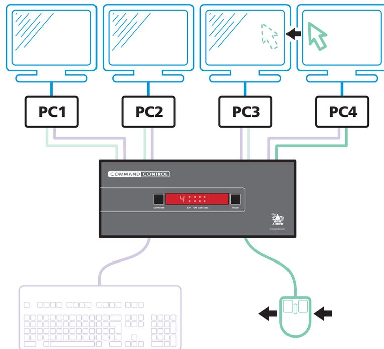
Free-Flow consists of special code within the CCS4-USB unit plus an intuitive graphical configuration application. First you inform the Free-Flow configuration application how many screens you have, their pixel resolutions and how they are physically arranged (e.g side-by-side, vertical stack, square formation, etc.). You then download this information to the CCS4-USB unit and this is used during operation to determine the precise moment to switch from one screen/system to the next.
