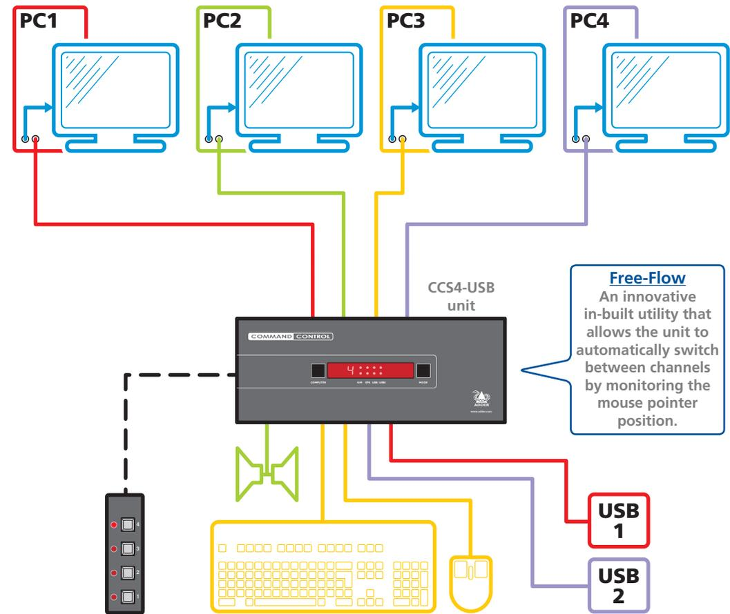
The optional remote control allows the CCS4-USB unit to be neatly concealed amongst the cabling.
