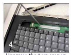
Unscrew the two screws on DDH holder
