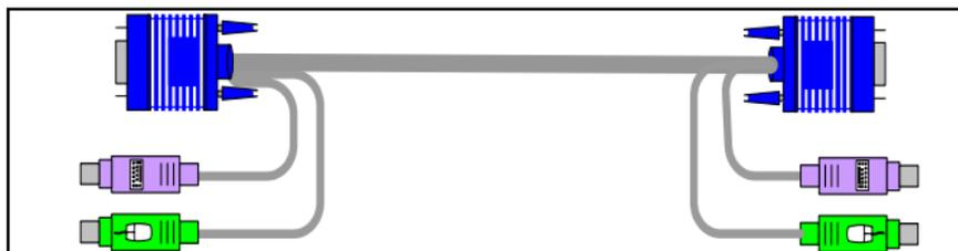
Figure 5 The 3 in 1 CPU cable
