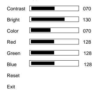
Use the +and – buttons to choose the desired parameter, press Menu to select and then use + or – to increase or decrease the value. Press Menu to save the value. When finished with all adjustments, use the + and – buttons to move to Exit and then press Menu to actually exit the routine.
