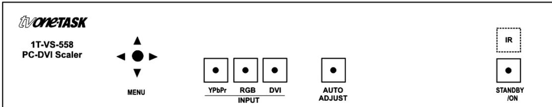
Above the word “MENU” you’ll find a joystick/switch control that allows access to and adjustment of various operational items. Pressing the top of the joystick will bring up the menu On Screen Display (OSD) and moving the joystick will allow you to move to, select and then adjust the various functions.
