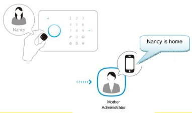
Remark : Users can only receive a notification if a mobile-number is stored and the RFID-tags have a name stored.
